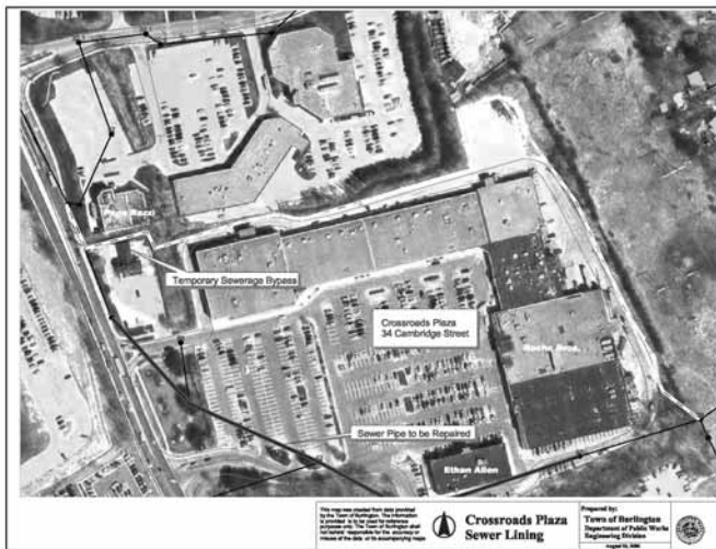
Crossroads Lining Project – Sewerage Bypass Plan
