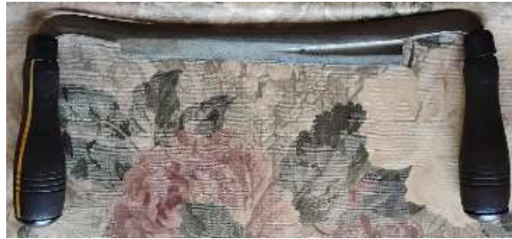
Bennet family drawknife showing extensive wear over three generations of use
