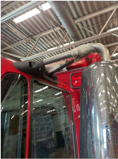
Drivers side mirror held together by tape. Mirrors are discontinued and are no longer available.
