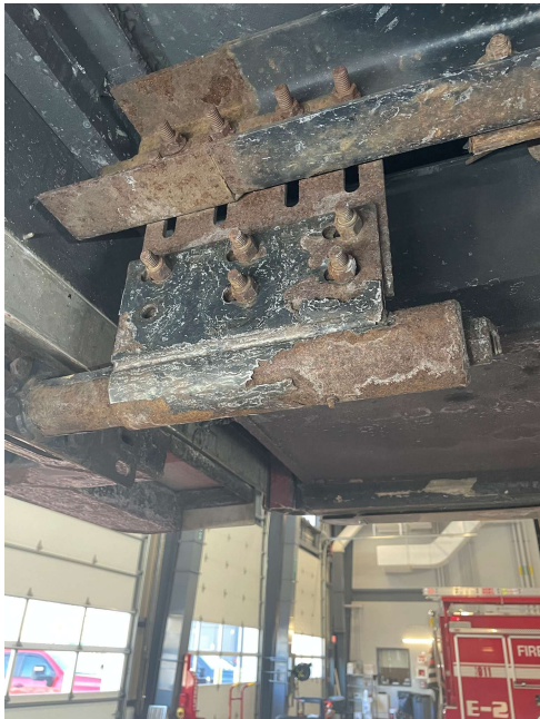
1 of 2 rear crash supports. Both are badly rotted and these parts are discontinued.
