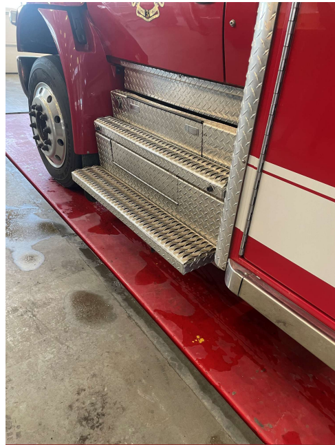
Frame that the step is bolted to is rotted, causing the step to be dangerously loose.
