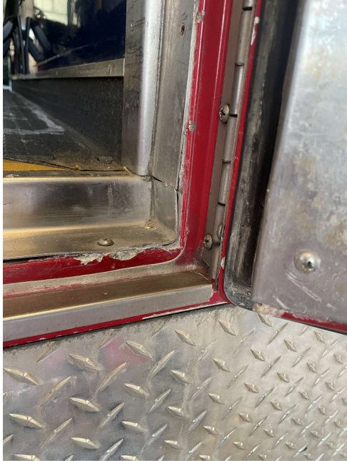
The floor is delaminated and is lifting the stainless trim plate. Doesn't close well.
