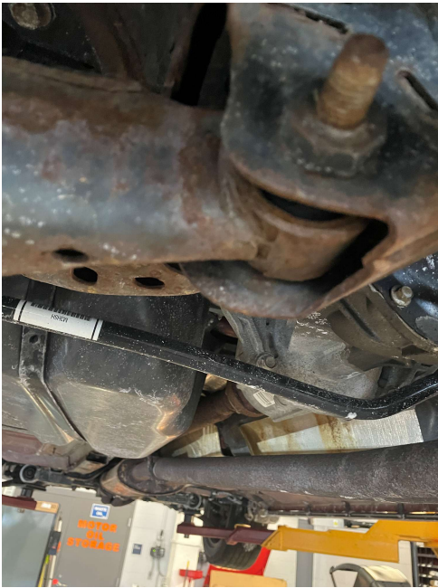
Right rear control arm. This is starting to rot.
