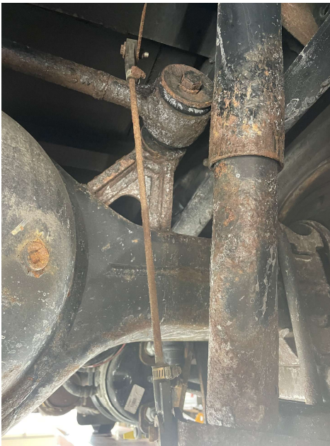
Leveling and the anti-sway bars. Rot and delamination.
