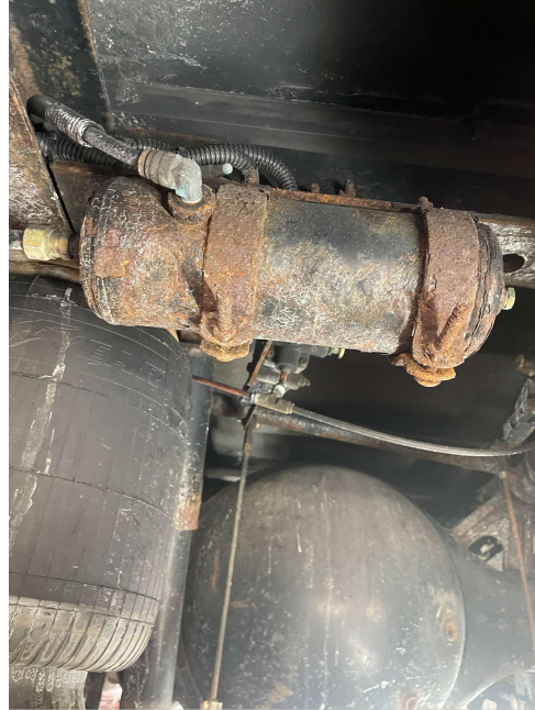
1 of 2 reserve air tanks for the rear suspension. Both are rotted and no longer available.
