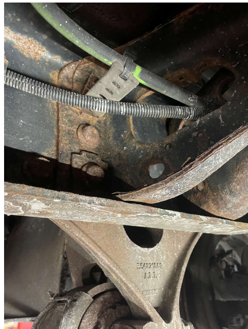
Structural cross-member above the transmission. Showing signs of delamination.
