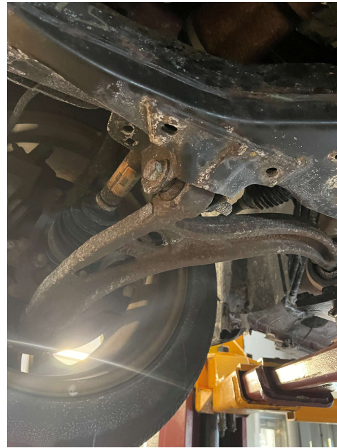
Left rear control arm. Badly rotted.
